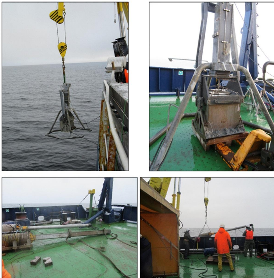
Fig. 2. The box corer (50x50x60 cm, Oktopus 2500, Oktopus GmbH, Kiel, Germany) allows for an undisturbed sampling of near-surface sediments of 0.25 m 2 and a downcore penetration of max. 50 cm (upper panel). Long sediment cores (lower panel) were obtained by a the gravity corer (3 - 5 m long steel barrel with liner, diameter 12 cm, head weight up to 1 t, GC 125, Oktopus GmbH, Kiel, Germany) and a square-barrel gravity corer (15x15 cm, 3 m, HYDROWERKSTAETTEN, Kiel, Germany).
